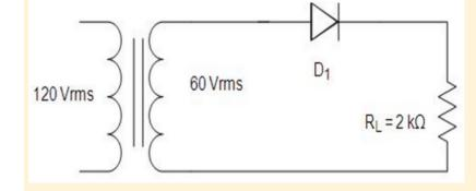
i. The output voltage. ii.Average voltage of the circuit
