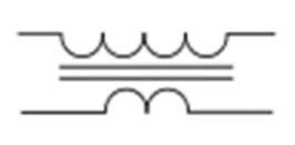
Fig 5:Step-down or step-up transformer.
