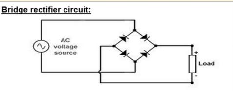
Fig 17:Bridge rectifier circuit diagram.
