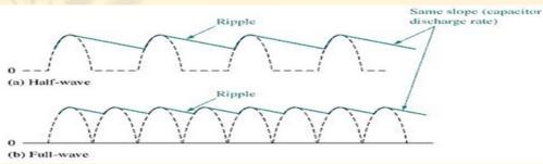
Fig 22:The ripple output at (a) Half-wave and (b) Full-wave rectifier
