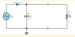
Fig 23:Capacitor Filter
