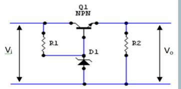
Fig 32:The Serial Transistor Regulator circuit
