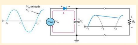
Fig 26:The capacitor charges back to peak of input when diode becomes forward-biased.
