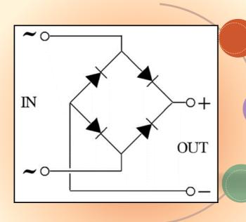
Bridge rectifier is also available in special packages containing the four diodes required.
