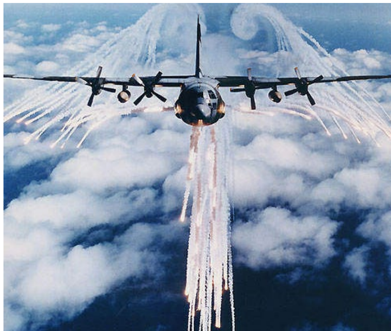
Figure 19: Chaff Flare to Protect Aircraft from Missile Radar
