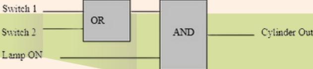
Figure 3.3: Example of function block diagram
