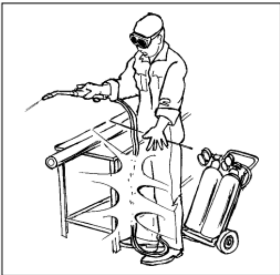
Flashback can result in the hose exploding, and/or catching fire. In extreme cases, the regulator may catch fire.
