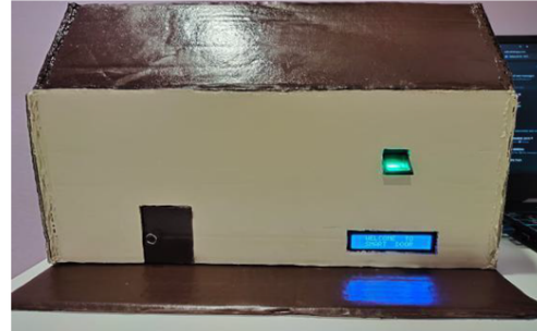
Figure 1: Unlocking the door using the fingerprint
