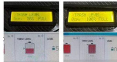
Figure 1: Dustbin volume readings on LCD and IOT applications.
