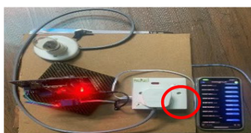
Figure 2: The led indicate the socket is off
