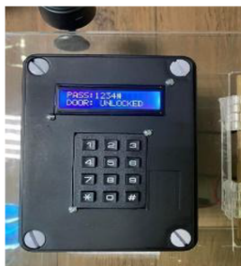
Figure 1: Shows the password that has been entered by the keypad to unlock the door.
