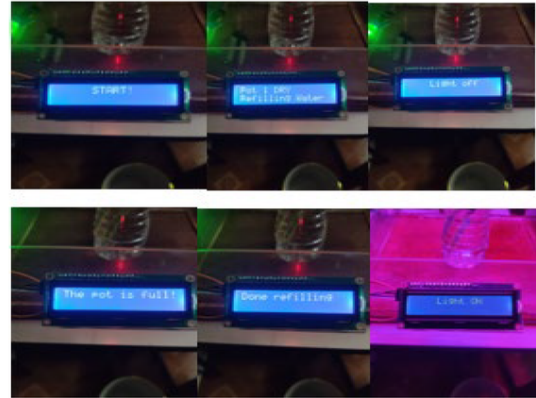
Figure 2: Results shown in LCD screen
