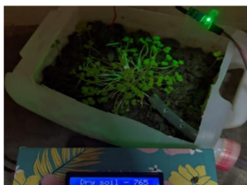
Figure 1: Soil value in dry condition is 765
