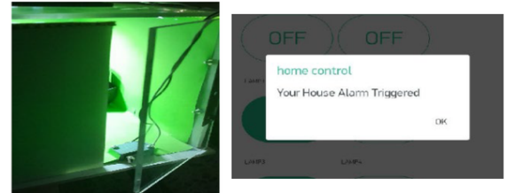
Figure 2: The alert notification in mobile when the door is open monitored by android
