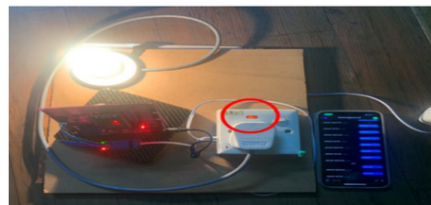
Figure 3: The command receive from telegram and led indicate the socket is on
