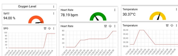
Figure 1: MQTT dashboard data displays for oxygen saturation (SpO 2 ), heart rate (BPM), and temperature.
