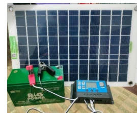
Figure 2: Solar, Battery, Solar Charge Controller
